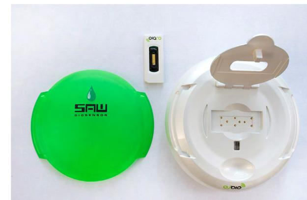
*OJ-Bio’s prototype medical diagnostic device, showing the disposable biochip on which the test sample is placed. Credit: OJ-Bio*
